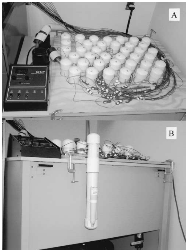
Fig. 1. Refrigerated bath modified for use with Cone-tainers. Plastic tubes were glued to a plywood frame (A). A mock tube was supported next to the bath to show Cone-tainer depth after placement inside the tube (B).
